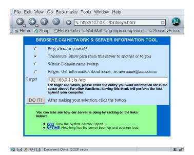
Figure 4. Web based network diagnostic utility
