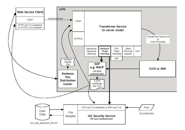
The logical structure of the Artix Advanced for z/OS Transformer server [2] is shown in figure 2. This server is the component in Artix Advanced for z/OS which provided Web Service integration between SOAP based client programs in the CICS and IMS transaction systems on the mainframe. This figure shows that the client and server both communicate with the KDC to obtain tickets, and that the client then sends the ticket with the SOAP request, which is, in turn, authenticated by the server.
