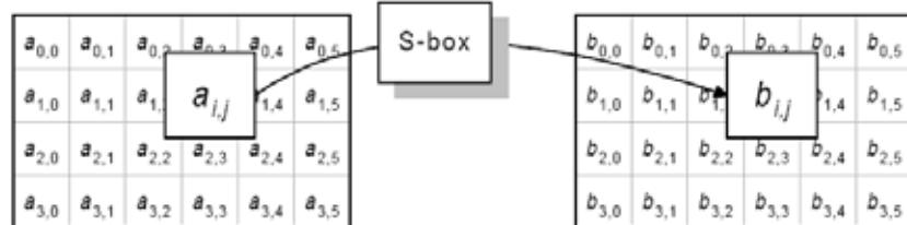
Figure1. Byte Substitution through S-box
