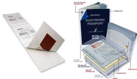
Figure 1: RFID tags embedded in a shipping label and a passport [4].
