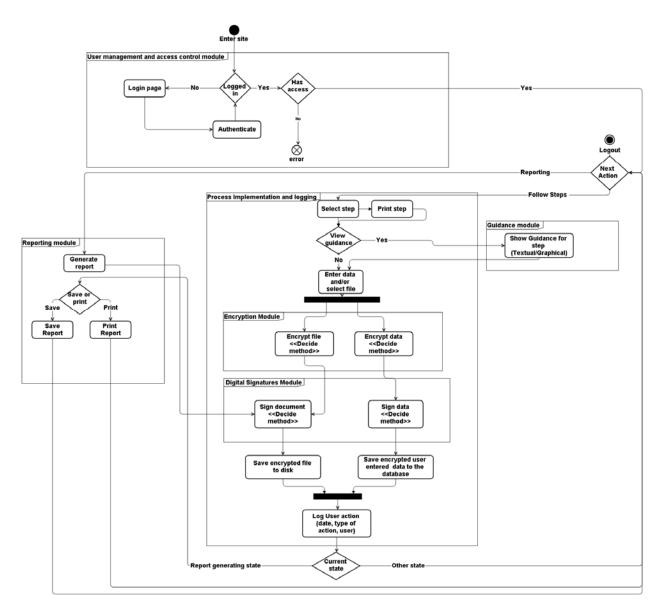
Figure 4: Prototype component activity diagram
